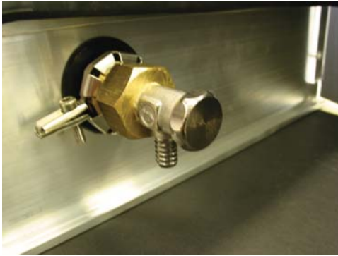
Exhauster completely mounted . All other connections as well as the covers are mounted in the same way.
